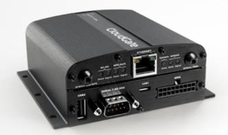
The Telematics Card allows the CloudGate Intelligent M2M Gateway to be used in advanced industrial telematics applications. The board can accept a range of Option or 3rd party developed I/O expanders that match the card and I/O connector to specific applications.
