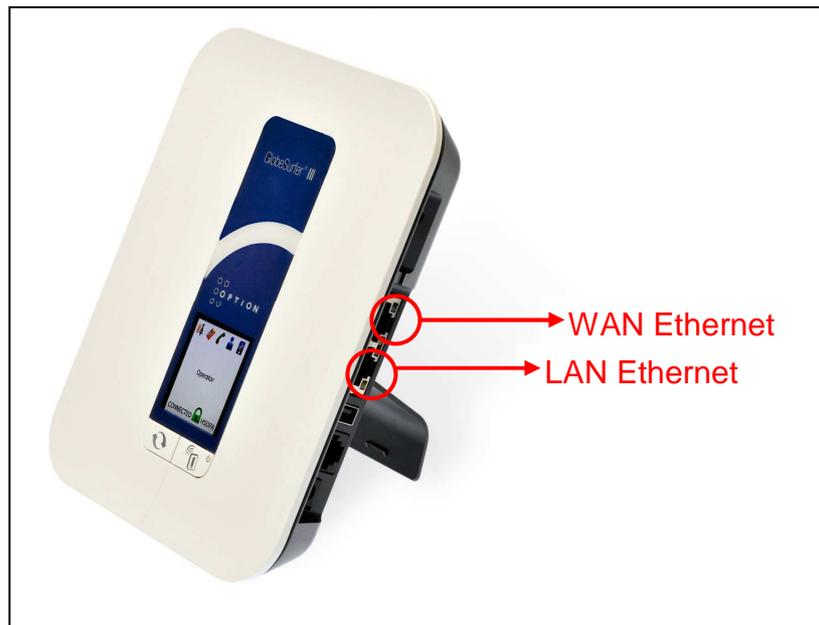
**Figure 6: LAN Ethernet and WAN Ethernet interfaces on the GS3.**
